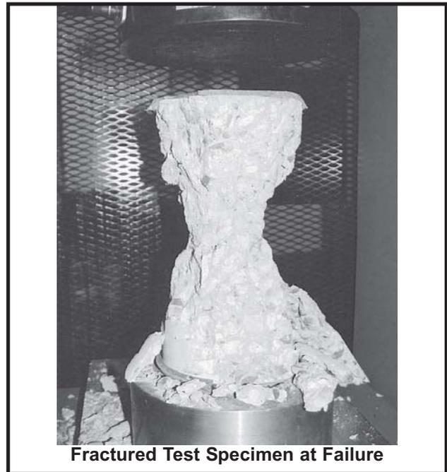
Fractured Test Specimen at Failure
